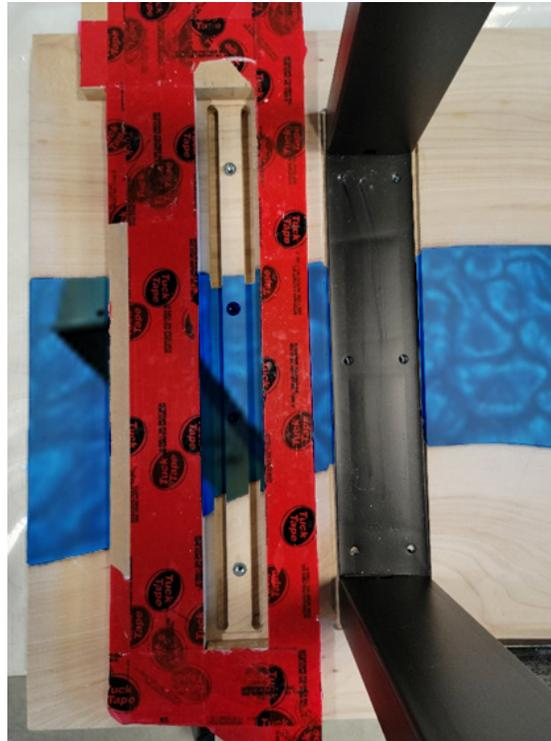
Figure 26: Fixture setup for c-channel
