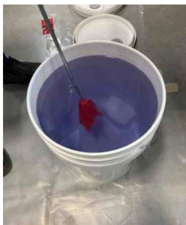
Figure 5: Mixing FlowCast Part A and B
