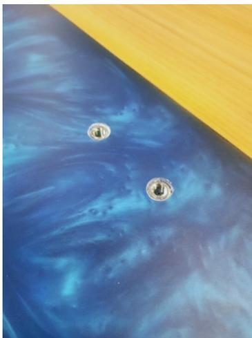
Figure 22: Inserts installed
