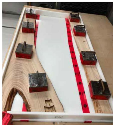
Figure 3: Test fitting wood slabs in mold
