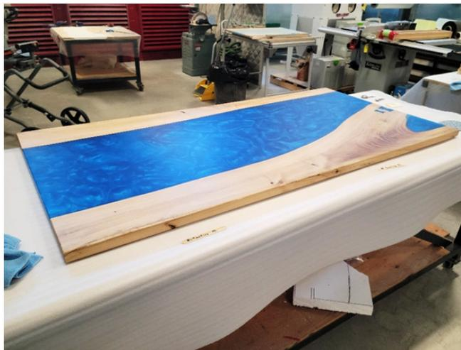
Figure 19: Table after 2 coats of Rubio Monocoat
