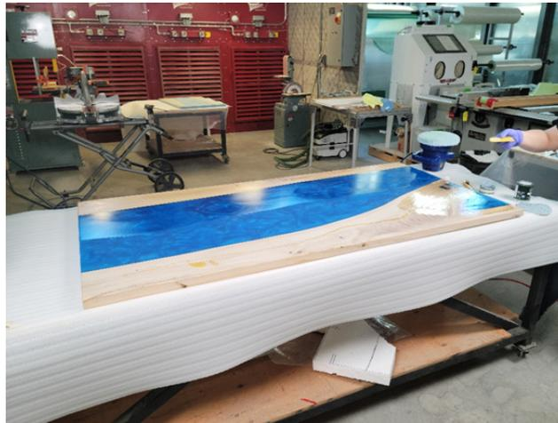
Figure 18: Application of Rubio Monocoat
