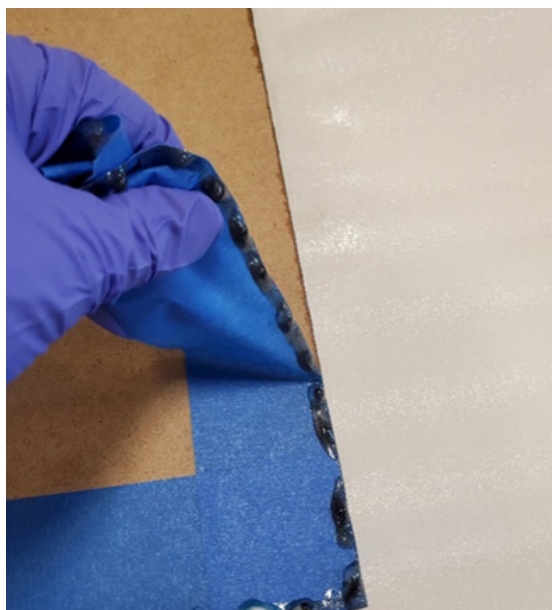
Figure 17: Peeling off the tape and resin drips
